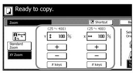
**3** Press [+] and [–] to set the *X* and *Y* zoom ratios. Press [# keys] ([#-Keys]) to enter with numeric keys.
